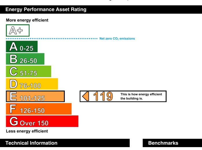
Main heating fuel:Grid Supplied ElectricityBuilding environment:Air ConditioningTotal useful floor area (m²):905Building complexity (NOS level):4Building emission rate (kgCO2/m²):151.9
