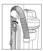
Twist the quick release the power cord.
