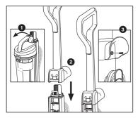
Remove the dust canister before installing handle. Push the handle onto the vacuum body, and use a Phillips screwdriver to secure it with the screw provided. IMPORTANT: The handle must be inserted first before replacing dust canister.
