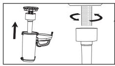
7. Lift out the assembly from transparent dust canister, and then untwist filter from the central tube to remove for cleaning dirt and debris as needed. Follow steps in reverse to reassemble.
