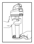
Hold dust canister over rubbish bin and unclip the lock on the bottom of the canister, allowing the dust to empty.
