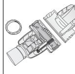
1. To release the turbo 2. Pull up on the plastic 3. Remove plastic upper upper cap of the pet cap and clean, removing pet hair and debris.
