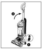
Step on the brush cover and pull back on handle, to engage button to switch for operation.
