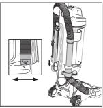
Place the short hose end onto the connector into the connector, and release cord hook to (left hand side if looking at the back of the vacuum), and rotate clockwise to lock.
