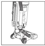
Push the hose handle place the 3-in-1 attachment onto the storage holder in front of the hose handle.
