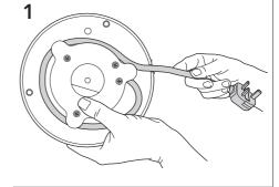
**2.** Fit the power cable firmly into the base slot so it is stable.
