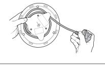
2. Fit the power cable firmly into the base slots,
