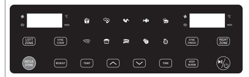
3.Press the TEMP button to enter temperature setting mode. Use the and buttons to adjust the temperature. Press the TIME button to enter time setting mode. Use the and buttons to adjust the time.
