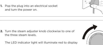
2. Turn the steam adjuster knob clockwise to one of the three steam levels. The LED indicator light will illuminate red to display that the appliance is heating. After around 30 seconds the light will turn green, indicating that the appliance is ready to use. **3.** Place the mop on the floor you wish to clean and tilt the handle back 45
