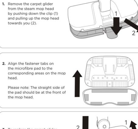
3. To replace the carpet glider, hook the front of the mop head under the lip of the carpet glider and push down so the clip clicks shut.
